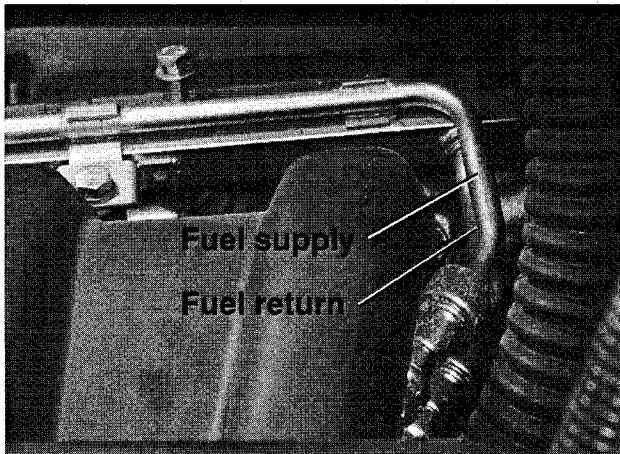
Fig. 14. Fuel lines at rear of intake manifold on M52 engine. Use BMW special tool 16 1 050 to release fittings.
