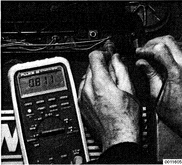
Fig. 14. Voltmeter connected across fuel injector connector with engine running. M50 engine shown.
