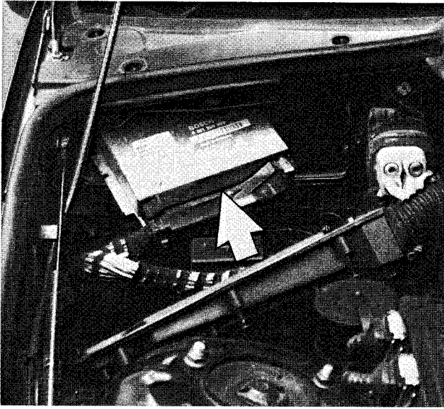
Fig. 42. Engine control module (ECM) located in compartment in right-rear of engine compartment (arrow).
